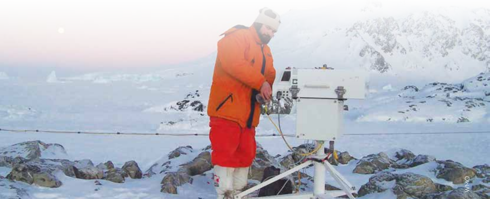
Total ozone measurement with a Brewer spectrophotometer at the Argentinian station of San Martin (68.1° S, 67.1° W)
